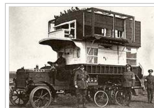
A B-type bus from London converted into a pigeon loft for use in northern France and Belgium during the First World War
